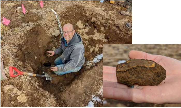
Left: Andy Gallagher, clearly happy with himself and collecting material from below the indurated horizon at the bottom of the pit. Right: What the indurated material looks like. Note the abrupt contact evidenced by the fine-grained yellow volcanic ash.
