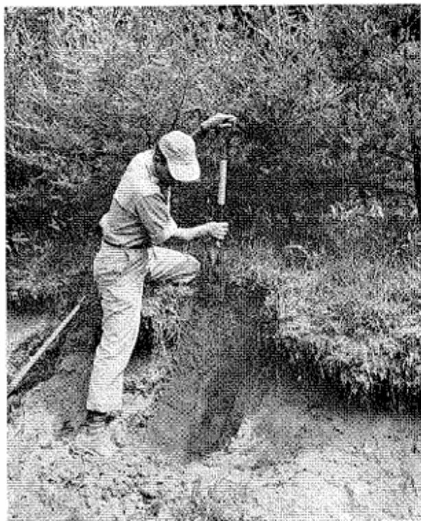
1. Dig a pit 4 by 4 feet and as deep as necessary to get the soil profile. A road cut may be selected but much care must be taken to insure an undisturbed profile. Above picture shows how cut or side of pit should be smoothed with "sharp shooter" or flat face spade.
