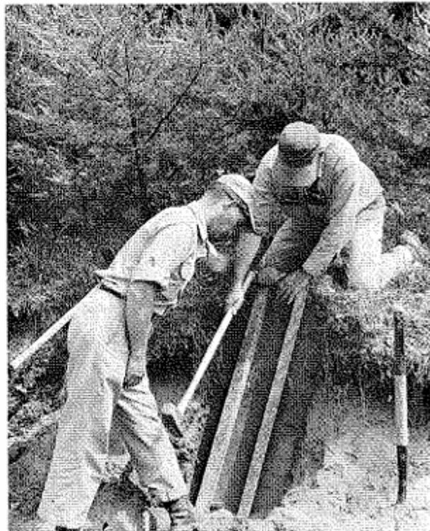
2. Steel sampling frame (monolith sampler) being driven into side of cut with sledge hammer. If soil is very hard or contains gravel, mark soil by running knife along side of frame. Cut around this marked area so that frame may be forced over cut.
