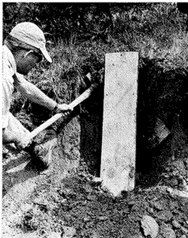
4. After cover board (10" x 48" x 1") has been bolted onto face of frame, use care not to loosen frame around soil. Dig soil away from sides of frame and cut soil behind the frame with sharp shooter. All roots must be cut. When they are fairly large, use pruning saw to cut them.
